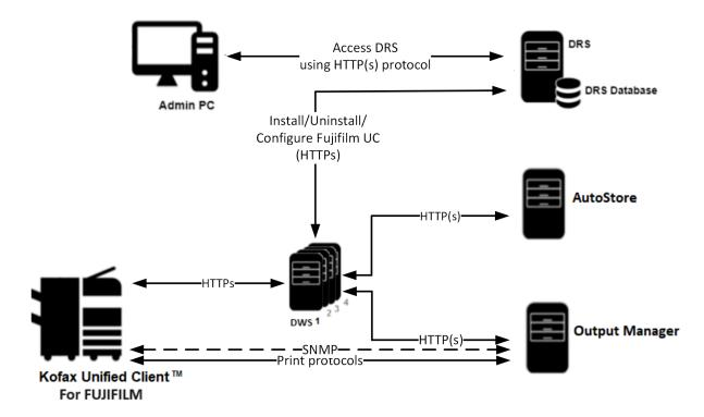
The Unified Client provides device authentication to securely access the device. It provides a single application for Kofax print and capture workflows.
