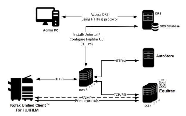
This figure illustrates a typical architecture for a system that includes the Unified Client for Fujifilm with Output Manager and AutoStore:
