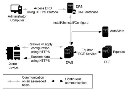
When used in an Output Manager configuration, the Unified Client for Xerox connects with the rest of ControlSuite as shown.
