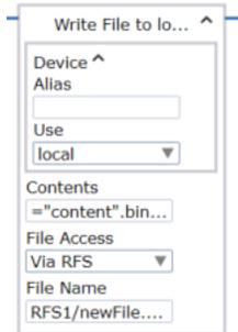
**Contents:** Specify a binary variable containing data to write to the Robot File System. In this example, "content" is the string written in the file. The file content must be binary.
